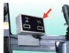
2 dimensional electric angle indicator
